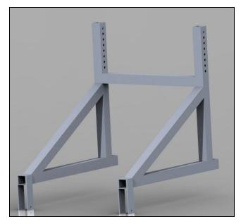
The bottom frame of the NewWalk is a single, welded component. This is the biggest and most sturdy component of the walker which is comprised of aluminum.
