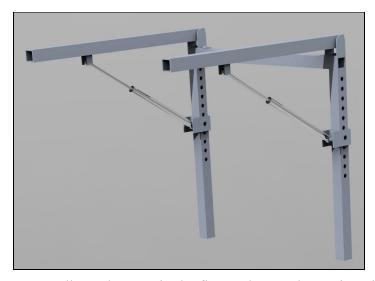
The top frame of the NewWalk can be seen in the figure above. The conjunction between the horizontal and vertical piece was partly welded and put together by a machinist, so tampering is highly unrecommended. The gas shocks shown in the figure can be seen in further detail in 2.4 *Gas Shocks*.
